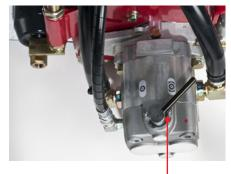
Reel Motor shut-off valve
