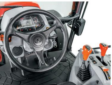
The handy steering wheel can be tilted forward when you exit the cab. Back in the seat, you can move it right back into its starting position. Simply press a pedal. Kubota has optimised the angle of the steering wheel, which gives you better visibility of the instrument panel and towards the front.
