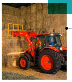
Whether you need to work with a manure fork, pallet fork, bale fork, or a bucket – each of them can be quickly attached and removed from the LA1854 front loader thanks to the standard EURO hitch interface.
